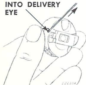
Fig. 20. Drawing the Thread Under the Tension Spring
