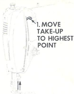
Fig. 14. Preparing for Removal of Bobbin
